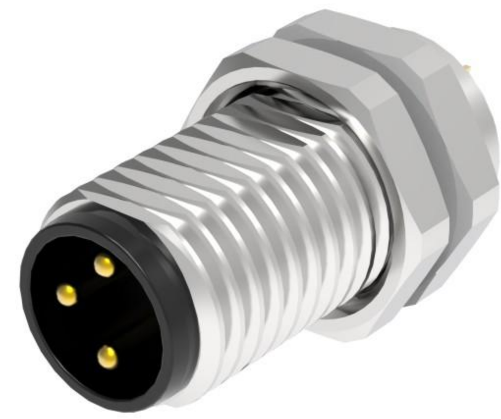
M8公头, 面板式连接器, 板后安装(锁板螺母M8*1.0), 焊杯式 M8 Male panel mount connector (panel nut M8*1.0) rear mounting, solder cup
