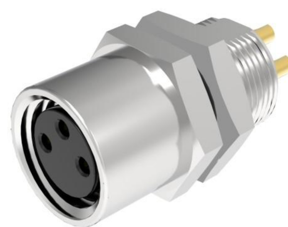
M8母头, 面板式连接器, 板前安装(锁板螺母M8*0.5)焊杯式 M8 Female panel mount connector, front mounting (panel nut M8*0.5) solder cup
