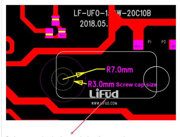
Safety standard of round aluminum substrate: 4.0mm (between screw cap margin and circuit wire)
