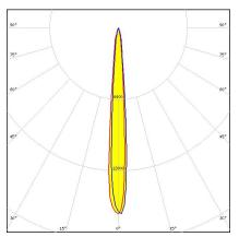
Dimensions: 16.1 mm x 16.1 mm Height: 9.50 mm ~14° spot beam optimized for Osram Oslon SSL80. Assembly with holder.
