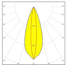
Dimensions: 16.1 mm x 16.1 mm Height: 9.30 mm ~35° + 15° oval beam optimized for Nichia NCSxx19. Assembly with holder, installation tape and location pins.
