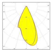
Dimensions: 16.1 mm x 16.1 mm Height: 9.70 mm ~45° wide beam optimized for CREE XP-E. Assembly with holder and installation tape.
