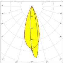
Dimensions: 16.1 mm x 16.1 mm Height: 9.70 mm Asymmetric beam for wall-washing.
