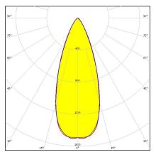
Dimensions: 16.1 mm x 16.1 mm Height: 11.00 mm ~46° wide beam optimized for Nichia NS6x83. Assembly with holder.
