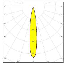
Dimensions: 16.1 mm x 16.1 mm Height: 9.65 mm ~16° diffused spot beam optimized for CREE XP-E. Assembly with holder.
