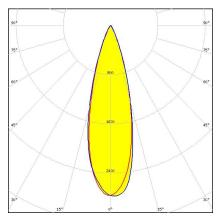
Dimensions: 16.1 mm x 16.1 mm Height: 9.65 mm ~30° medium beam optimized for CREE XB-D. Assembly with holder.
