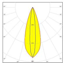
Dimensions: 16.1 mm x 16.1 mm Height: 9.65 mm ~35° + 15° oval beam optimized for CREE XB-D. Assembly with holder.
