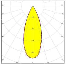
Dimensions: 16.1 mm x 16.1 mm Height: 9.65 mm ~45° wide beam optimized for CREE XB-D. Assembly with holder.
