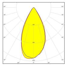
**Dimensions: 16.0 mm x 16.0 mm Height: 9.50 mm** ~45° wide beam optimized for CREE XP-E. Assembly with holder, installation tape and location pins.
