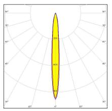
Dimensions: 16.1 mm x 16.1 mm Height: 9.50 mm ~16° diffused spot beam optimized for Osram Oslon SSL80. Assembly with holder.
