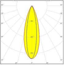
Dimensions: 16.1 mm x 16.1 mm Height: 11.00 mm ~35° + 15° oval beam optimized for
