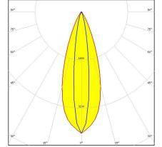
Dimensions: 16.1 mm x 16.1 mm Height: 9.82 mm ~35° + 15° oval beam optimized for CREE XP-E. Assembly with holder.
