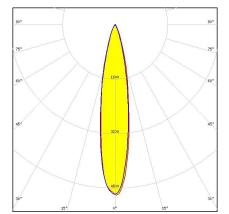
Dimensions: 16.1 mm x 16.1 mm Height: 11.00 mm ~14° spot beam optimized for Nichia NS6x83. Assembly with holder and
