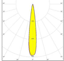
Dimensions: 16.1 mm x 16.1 mm Height: 9.65 mm ~14° spot beam optimized for CREE
