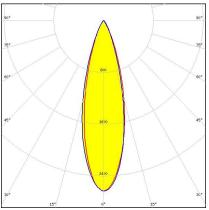
Dimensions: 16.1 mm x 16.1 mm Height: 9.30 mm ~30° medium beam optimized for Nichia
