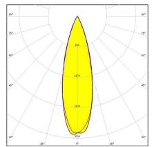
Dimensions: 16.1 mm x 16.1 mm Height: 9.70 mm ~30° medium beam optimized for CREE XP-E. Assembly with holder and installation tape.
