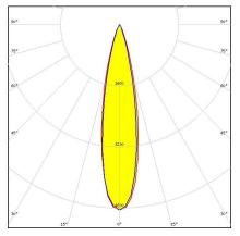
**Dimensions: 16.0 mm x 16.0 mm Height: 9.26 mm** ~20° smooth spot beam. Assembly with holder, installation tape and location pins.
