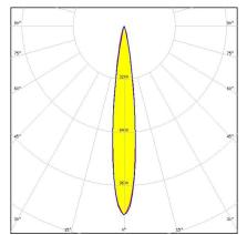
Dimensions: 16.1 mm x 16.1 mm Height: 9.50 mm ~14° spot beam optimized for Avago
