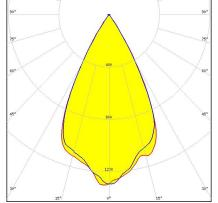
Dimensions: 16.1 mm x 16.1 mm Height: 9.65 mm ~45° wide beam optimized for CREE XP-E. Assembly with holder.
