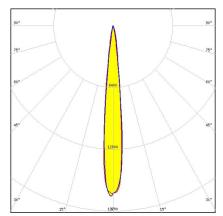
Dimensions: 16.1 mm x 16.1 mm Height: 9.70 mm ~14° spot beam optimized for CREE XP-E. Assembly with holder and installation tape.
