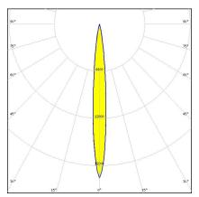
Dimensions: 67.0 mm x 67.0 mm Height: 11.10 mm ~14° spot beam
