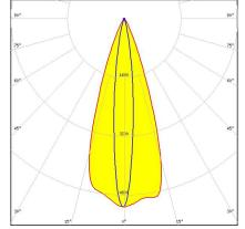
Dimensions: 26.0 mm x 26.0 mm Height: 16.20 mm ~35° + 8° oval beam. Assembly with installation tape.
