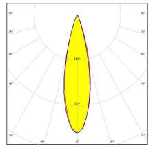
Dimensions: 26.0 mm x 26.0 mm Height: 16.70 mm ~25° medium beam. 16.7 mm high assembly with installation tape.
