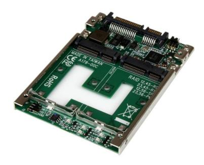
Vastly increase system performance by adding a dual mSATA SSD RAID array into any 2.5" SATA HDD application with the 25SAT22MSAT mSATA to SATA adapter.
