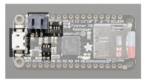
The above shows the Micro USB jack (left), Lipoly JST jack (top left), as well as the 3.3V regulator and changeover diode (just to the right of the JST jack) and the Lipoly charging circuitry (to the right of the Reset button). There's also a **CHG** LED, which will light up while the battery is charging. This LED might also flicker if the battery is not connected.
