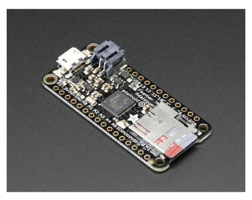
At the Feather M0's heart is an ATSAMD21G18 ARM Cortex M0 processor, clocked at 48 MHz and at 3.3V logic, the same one used in the new Arduino Zero (http://adafru.it/2843). This chip has a whopping 256K of FLASH (8x more than the Atmega328 or 32u4) and 32K of RAM (16x as much)! This chip comes with built in USB so it has USB-to-Serial program & debug capability built in with no need for an FTDI-like chip.
