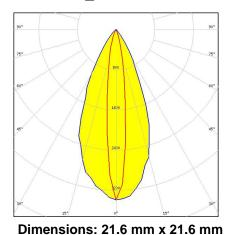
Height: 12.10 mm ~13° x 45° oval beam optimized for Cree XP-G and XP-E. Variant with beam direction rotated 90°.
