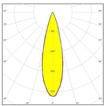
Dimensions: 21.6 mm x 21.6 mm Height: 11.70 mm ~25° medium beam
