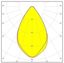
Dimensions: 50.0 mm x 50.0 mm Height: 8.50 mm ~65° wide beam optimized for CREE XP-L and XM-L
