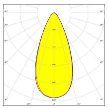
Dimensions: 50.0 mm x 50.0 mm Height: 8.50 mm ~50° wide beam. Variant made from PC.
