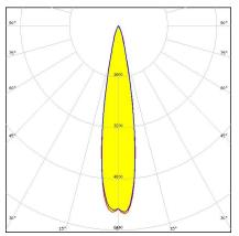
Dimensions: 50.0 mm x 50.0 mm Height: 10.00 mm ~10° spot beam
