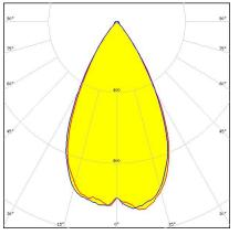
Dimensions: 50.0 mm x 50.0 mm Height: 8.50 mm ~50° wide beam optimized for CREE XP-L and XM-L
