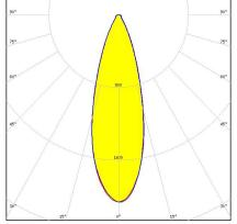
Dimensions: 50.0 mm x 50.0 mm Height: 8.50 mm ~25° medium beam optimized for CREE XP-L and XM-L
