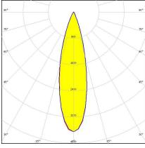
Dimensions: 50.0 mm x 50.0 mm Height: 8.50 mm ~25° medium beam
