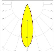
Dimensions: 50.0 mm x 50.0 mm Height: 8.50 mm ~25° medium beam optimized for CREE
