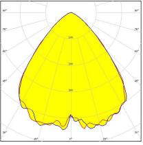
Dimensions: 25.0 mm x 25.0 mm Height: 9.81 mm ~90° beam
