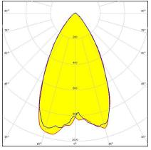
Dimensions: 25.0 mm x 25.0 mm Height: 9.81 mm ~60° beam
