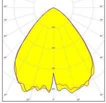
Dimensions: 25.0 mm x 25.0 mm Height: 9.96 mm ~90° beam. Assembly with installation tape.
