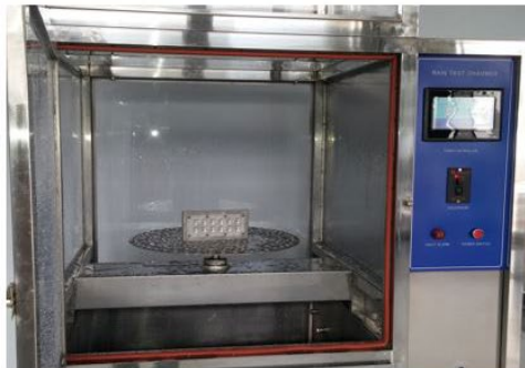
Testing under water jet
