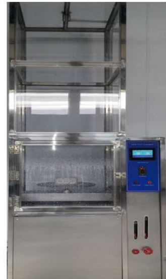
Testing under water jet
