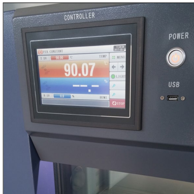
Temperature set in the climatic chamber
