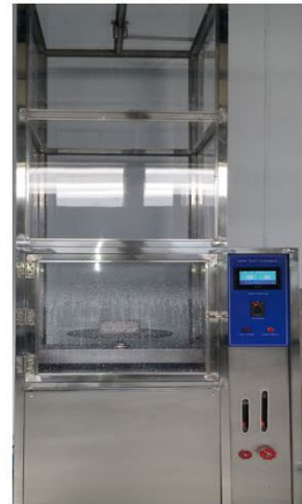
Testing under water jet
