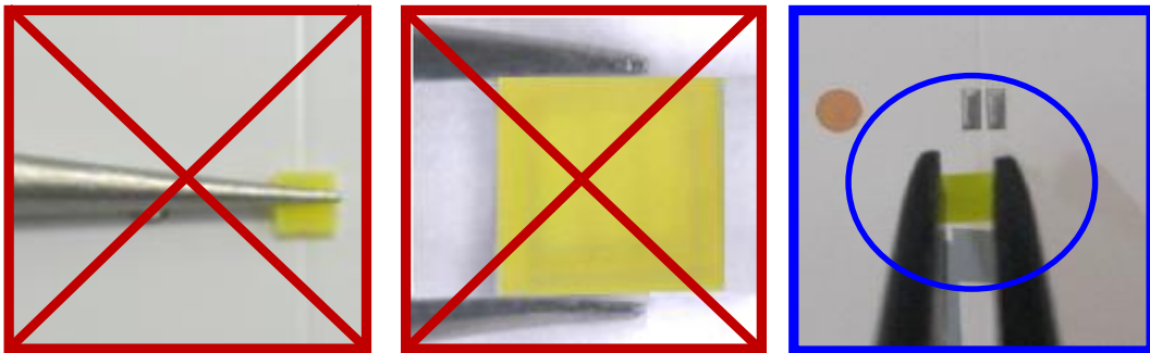
Figure 3 (a). Incorrect handling of WICOP LEDs
