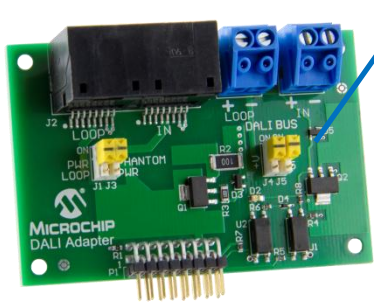
DALI Adapter with 2-wire & RJ45 connections
