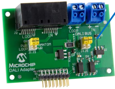
DALI Adapter with 2-wire & RJ45 connections
