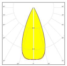
Dimensions: 50.0 mm x 50.0 mm Height: 17.00 mm ~50° wide beam Dimensions: 50.0 mm x 50.0 mm Height: 15.30 mm ~50° wide beam
