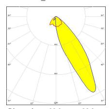
Dimensions: 32.0 mm x 32.0 mm Height: 20.75 mm Asymmetric beam for wall-washing. Assembly with holder and installation tape.
