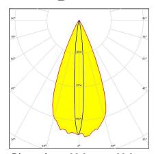
Dimensions: 32.0 mm x 32.0 mm Height: 19.05 mm ~20° + 40° oval beam. Assembly with holder and installation tape.
