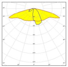
Dimensions: 25.0 mm x 25.0 mm Height: 8.60 mm IESNA Type II (medium) beam,
