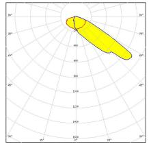
**Dimensions: 25.0 mm x 25.0 mm Height: 12.60 mm** Forward throw beam for area lighting. Assembly with installation tape.
