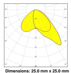
Height: 8.77 mm Beam for area lighting with shorter illumination distances. Optimized for CREE XP-G and XP-E.
