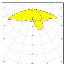
Dimensions: 25.0 mm x 25.0 mm Height: 9.10 mm IESNA Type II (medium) beam with minimized house side backlight. Version with location pins.
