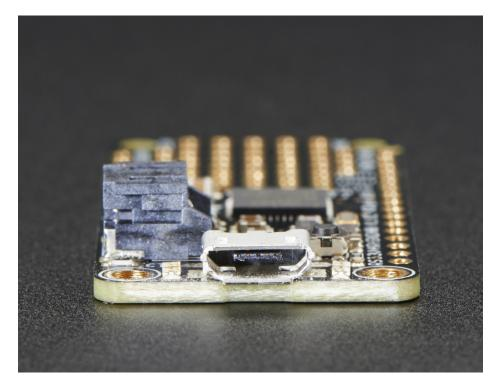
Comes fully assembled and tested, with a USB bootloader that lets you quickly use it with the Arduino IDE. We also toss in some header so you can solder it in and plug into a solderless breadboard. Lipoly battery and USB cable not included (but we do have lots of options in the shop if you'd like!)
