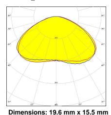
**Height: 5.70 mm**Beam for area and street lighting such as parks and pedestrian walkways. Lens with installation clips.
