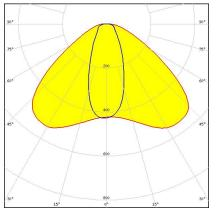
Dimensions: 19.6 mm x 15.5 mm Height: 5.20 mm Wide oval beam for area lighting
