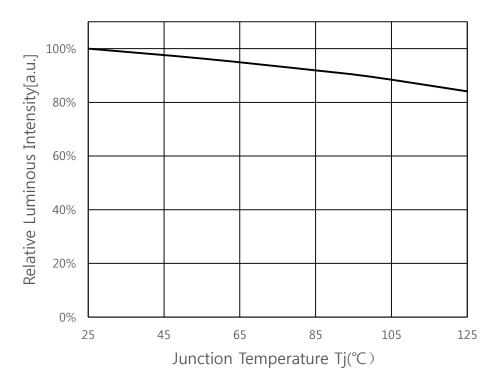
Fig 6. Junction Temperature vs. Relative Luminous Intensity,  $I_F$ =120mA
