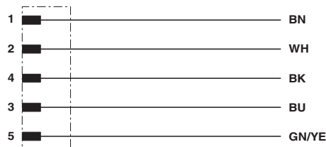
Contact assignment of the M12 plug
