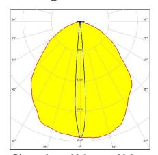
Dimensions: 33.9 mm x 33.3 mm Height: 16.90 mm 34 x 33 mm lens with ~100° x 15° oval beam. Assembly with installation tape.
