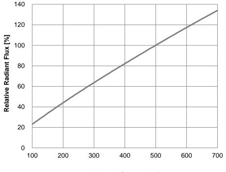
Fig 3. Forward Current vs. Relative Radiant Flux, T<sub>s</sub>=25°C
