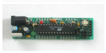
If you'd like to take advantage of the auto-reset capabilities added to the Arduino software, install ceramic capacitor **C6**.
