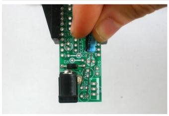
Next, its time to place the 25V electrolytic capacitor C3. Electrolytic capacitors are *polarized* which means they only work well in one direction. Put it in backwards and they can explode! You can tell how to place it because the silkscreened image has a plus near one hole and the capacitor has one long lead. That lead is the positive lead. In this image, its the one on the right.
