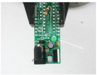
The 1K resistor **R2** goes in, its the LED's matching resistor. Bend it over as shown to place it.
