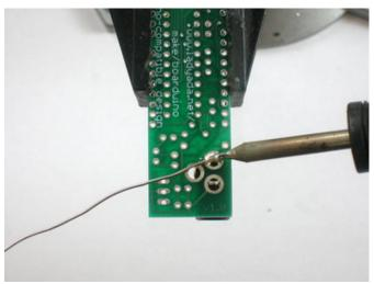
Use the soldering iron to heat up each of the 3 connections and poke the solder in so that it melts into the holes.
