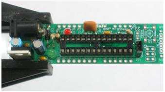
Place the 28 pin socket. This is to allow you to replace the microcontroller if necessary. Make sure the notch in the socket matches the notch in the silkscreened image. In this picture, its on the right.
