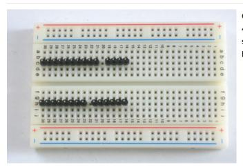
Cut 4 more pieces of header, a 10-pin, 8-pin, 6-pin and 4-pin. Insert them into a solderless breadboard as shown so that the long legs are in the solderless breadboard sockets.
