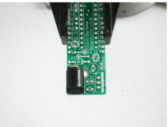
Place the 2.1mm DC jack as shown, it should fit in snugly. Make sure the part is on the top of the board, so that you can see the silkscreened images.
