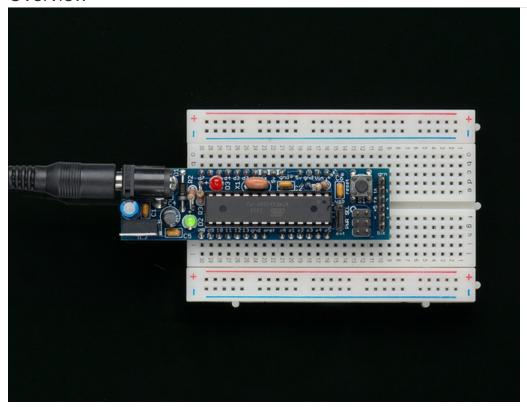
If you've ever struggled to use a solderless breadboard with an Arduino, you understand how frustrating it can be! I designed this Arduino clone to solve this problem in an inexpensive DIY fashion. Kits with all parts are available in the Adafruit webshop (https://adafru.it/aJD).
