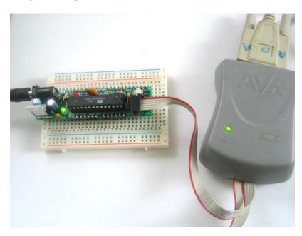
There is also a standard 6-pin ICSP (In-Circuit Serial Programming) cable that can be used to burn a new bootloader or just reprogram the chip.
