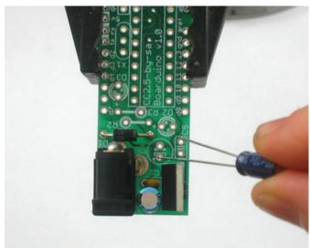
Now you should soder in the 6.3V electrolytic capacitor **C4** as shown. Remember its polarized so you must place the longer lead in the positive-marked hole.
