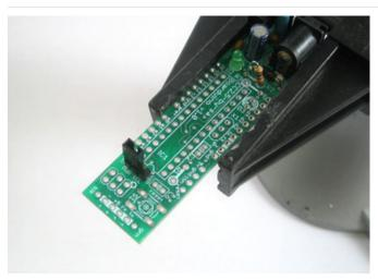
Place the jumper/shunt as shown, so that its on the **EXT** pair of pins.
