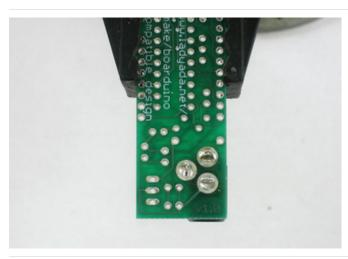
Make sure all three pads are soldered, with plenty of solder, the holes should be filled up. This gives the jack mechanical strength.
