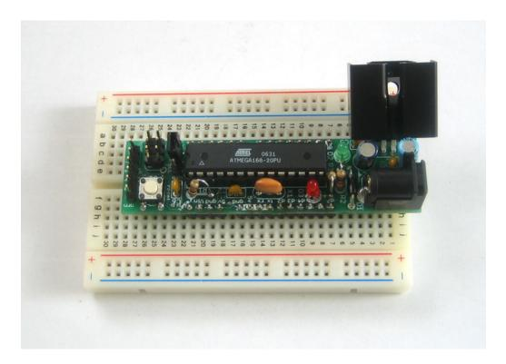
If you are planning to draw a lot of power from the 5V regulator, say for servos or many LEDs, you may want to add a heatsink to the 7805. Just bend the regulator back a bit and slip one on.
