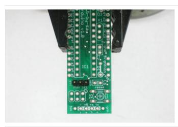
Place the 3 pin header at the other end of the board as shown. the short end goes into the PCB, and the long ends extend up.
