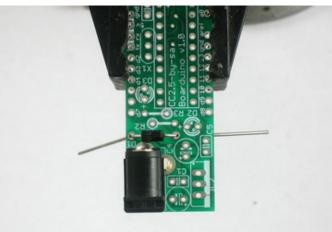
Next, place the 1N4001 diode **D1**. Diodes are directional, they only let current flow in one direction. This diode is used to protect the Boarduino from damage. Make sure the white stripe on the diode matches the white stripe in the silkscreened image below. In this picture, the stripe is on the right.
