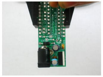
Next is the green 3mm LED **D2**. Like the electrolytic capacitors, LEDs have polarity and they wont work if soldered in backwards. The long lead is the positive lead, make sure it goes in the hole with a + next to it.
