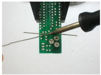
Turn the PCB over and solder both legs so that you get a nice shiny solder joint.
