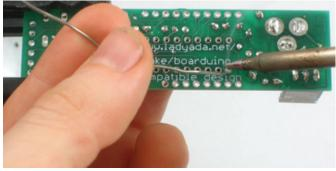
Solder in the socket by tacking two opposite corners and then soldering the rest of the pins. Press the socket into the board to make sure its flat up against it.
