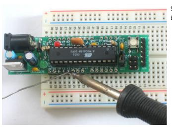
Solder all of the pins of the header, making sure that the board is sitting flat against the header.
