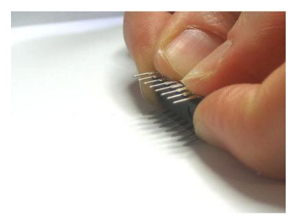
Once the pins are straight, insert the chip by matching the  ${\bf U}$  notch in the chip with the  ${\bf U}$  notch in the socket.
