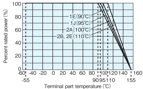
When the terminal part temperature of the resistor exceeds the rated terminal part temperature shown above, the power shall be derated according to the derating curve.
