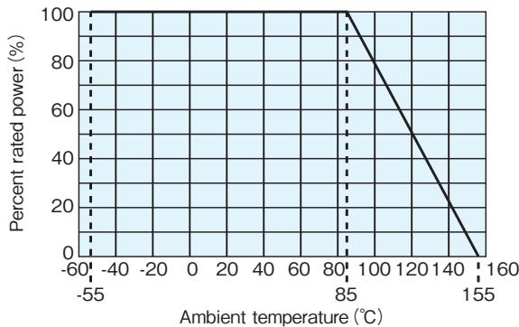
For resistors operated at an ambient temperature of 85°C or higher, the power shall be derated in accordance with the above derating curve.
