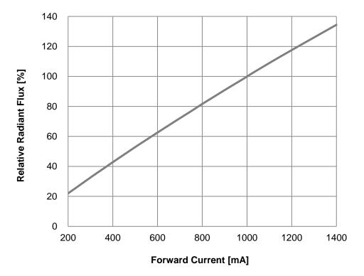
Fig 3. Forward Current vs. Relative Radiant Flux, T<sub>s</sub>=25°C
