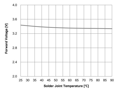
Fig 7. Solder Joint Temperature vs. Forward Voltage, I<sub>F</sub>=1A
