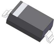
SOD-123 * Band marking denotes cathode
