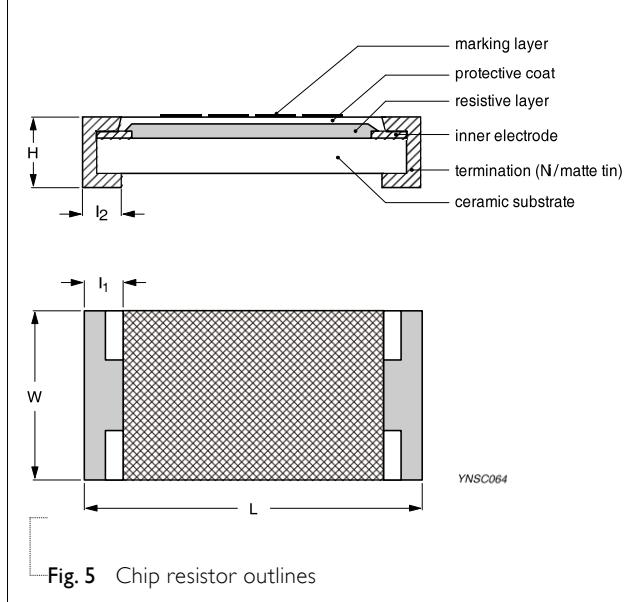
Fig. 5 Chip resistor outlines
