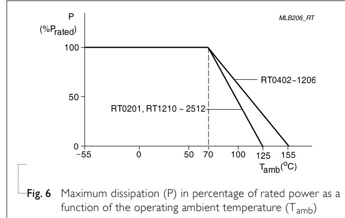
Fig. 6 Maximum dissipation (P) in percentage of rated power as a function of the operating ambient temperature ( $T_{amb}$ )
