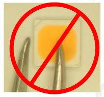
(2) In general, LEDs should only be handled from the side. By the way, this also applies to LEDs without a silicone sealant, since the surface can also become scratched.
