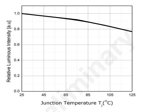
Fig 6. Junction Temperature vs. Relative Luminous Intensity,  $I_F$ =150mA
