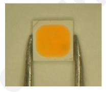
(3) When populating boards in SMT production, there are basically no restrictions regarding the form of the pick and place nozzle, except that mechanical pressure on the surface of the resin must be prevented. This is assured by choosing a pick and place nozzle which is larger than the LED's reflector area.
