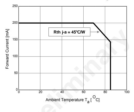
Fig 9. Ambient Temperature vs. Maximum Forward Current,  $T_{j_{max}}$  = 125°C
