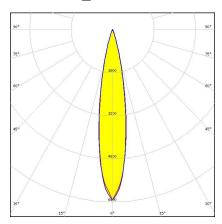
Dimensions: 38.0 mm x 38.0 mm Height: 29.60 mm ~25° medium beam with sublens
