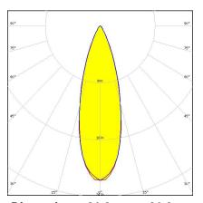
Dimensions: 21.6 mm x 21.6 mm Height: 12.90 mm ~30° medium beam optimized for LUXEON Rebel. Assembly with
