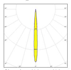
Dimensions: 21.6 mm x 21.6 mm Height: 12.90 mm ~8° spot beam optimized for LUXEON Rebel. Assembly with
