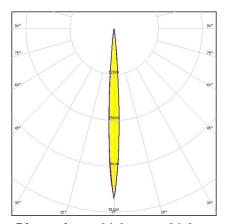
Dimensions: 21.6 mm x 21.6 mm Height: 13.10 mm ~8° spot beam optimized for CREE XP-E. Assembly with black holder
