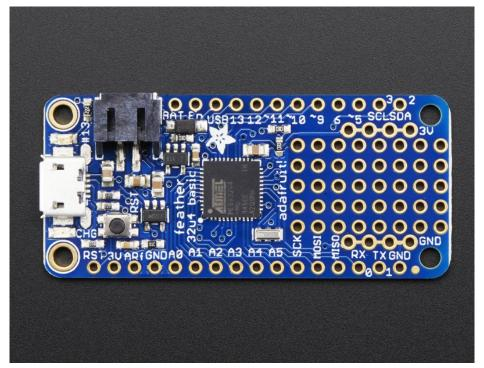
At the Feather 32u4's heart is at ATmega32u4 clocked at 8 MHz and at 3.3V logic, a chip setup we've had tons of experience with as it's the same as the Flora (https://adafru.it/dVI). This chip has 32K of flash and 2K of RAM, with built in USB so not only does it have a USB-to-Serial program & debug capability built in with no need for an FTDI-like chip, it can also act like a mouse, keyboard, USB MIDI device, etc.
