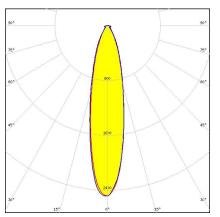
Dimensions: 38.0 mm x 38.0 mm Height: 11.40 mm ~20° medium beam
