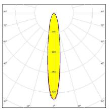
Dimensions: 38.0 mm x 38.0 mm Height: 10.60 mm ~19° spot beam
