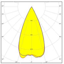
Dimensions: 50.0 mm x 50.0 mm Height: 25.45 mm ~55° wide beam. Assembly with holder C
