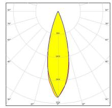
Dimensions: 50.0 mm x 50.0 mm Height: 25.45 mm ~35° medium beam. Assembly with holder C compatible with LEDiL HEKLA.
