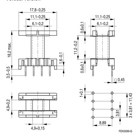
Hole arrangement View in mounting direction
