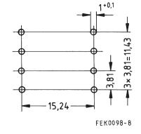
Hole arrangement View in mounting direction
